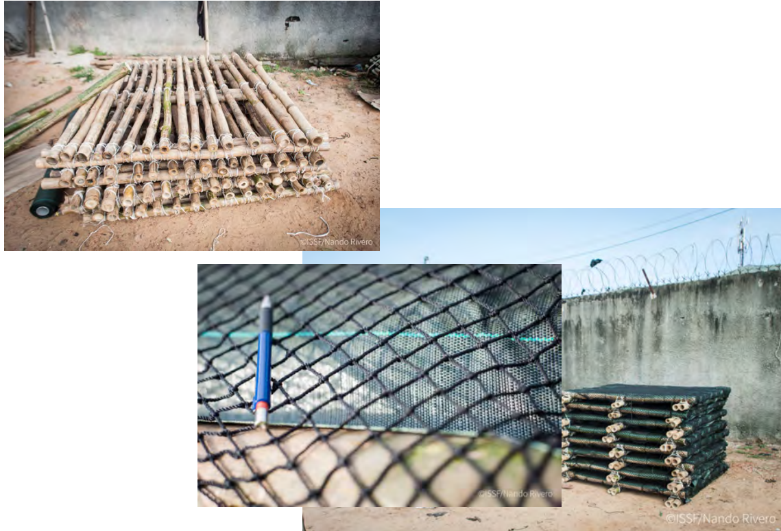
Figure 5. Bamboo canes used in the raft, covered with low entanglement risk black plastic net
